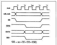
Figure 12: Read Cycle Timing.
