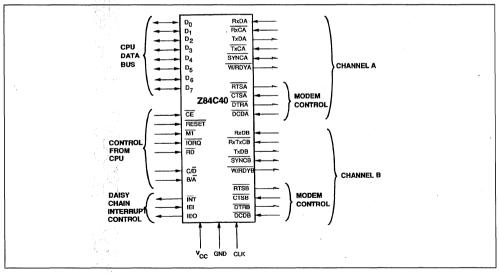
Figure 6 : Z80C SIO-0 Dual in Line Pin Configuration.
