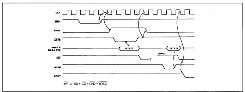
Figure 16: Mode 3 Bit Mode Timing.
