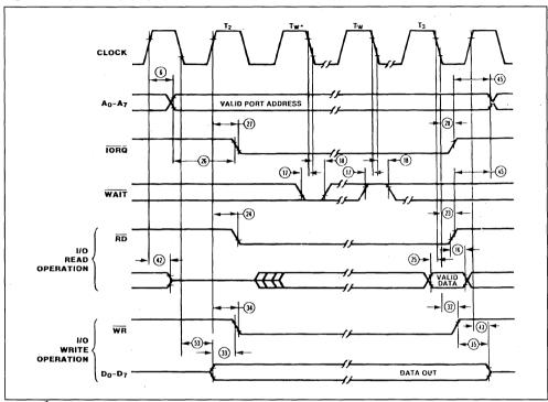
Note: Tw\* = One Wait cycle automatically inserted by CPU.
