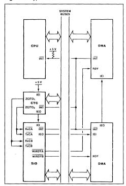
the system buses are released to the CPU. The buses are requested again for each succeeding byte operation.
