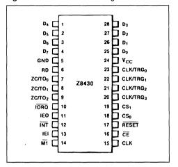
Figure 2: Chip-Carrier Pin Configuration.
