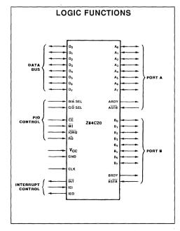
Figure 1: Dual in Line Pin Configuration.
