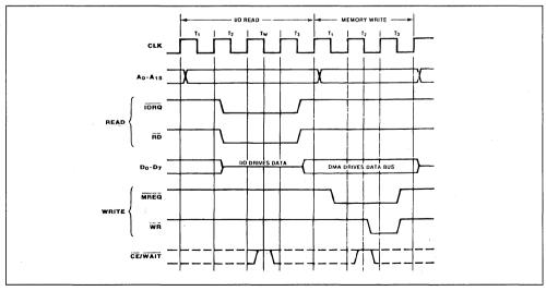
(figure 18). The action on BUSREQ is thus somewhat delayed from action on the RDY line. The DMA always completes its current byte operation in an orderly fashion before releasing the bus.
