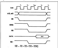
Figure 13: Mode 0 Output Timing.
