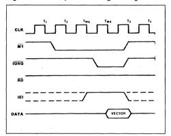
daisy chain enable lines for proper control of nested priority interrupt handling. The CTC decodes the 2-byte RETI code internally and determines whether it is intended for a channel being serviced. Figure 15 shows RETI timing.
