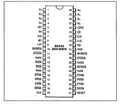
TxDA and TxDB marking, forces the modem controls High and disables all interrupts. The control registers must be rewritten after the SIO is reset and before data is transmitted or received.
