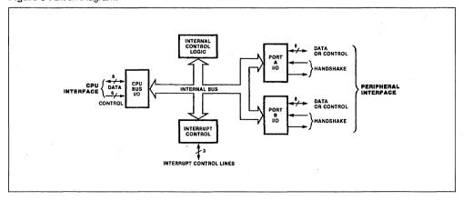
Figure 4: Typical Port I/O Block Diagram.
