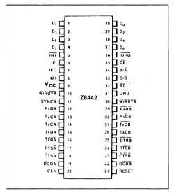
SIO is programmed for Auto Enables; otherwise they may be used as general-purpose input pins. Both pins are Schmitt-trigger buffered to accommodate slow-risetime signals. The SIO detects pulses
