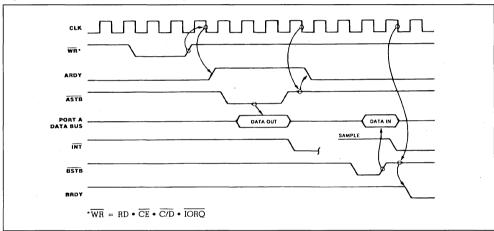
Figure 16: Mode 3 Bit Mode Timing.
