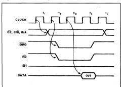
places its interrupt vector on the data bus and sets its internal interrupt-under-service latch.
