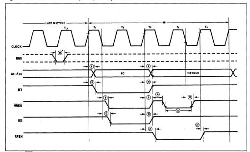
Although  $\overline{\text{NMI}}$  is an asynchronous input, to guarantee its being recognized on the following machine cycle, NMI's falling edge must occur no later than the rising edge of the clock cycle preceding T<sub>LAST</sub>.
