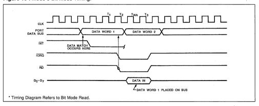
Figure 17: Interrupt Acknowledge Timing.
