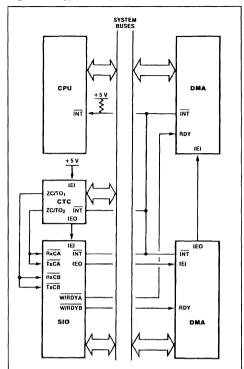
In all modes, once a byte of data is read into the DMA, the operation on the byte will be completed in an orderly fashion, regardless of the state of other signals (including a port's Ready line).
