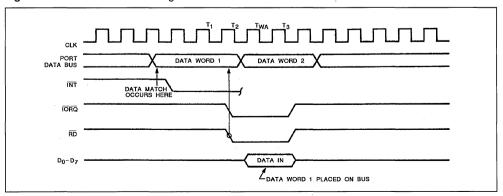
Figure 17: Interrupt Acknowledge Timing.
