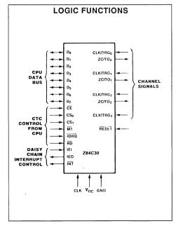
Interrupt processing is simplified because only one vector need be specified; the CTC internally generates a unique vector for each channel.
