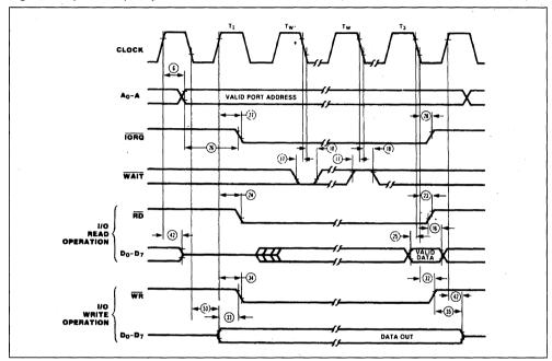
Note: Tw\* = One wait cycle automatically inserted by CPU.
