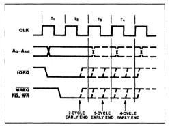
Figure 16: Bus Release (Byte-at-a-Time-Mode).
