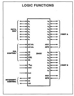
Figure 1: Dual in Line Pin Configuration.
