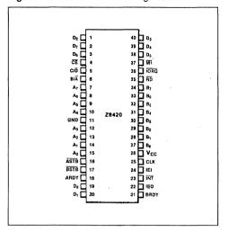
Figure 2: Chip Carrier pin Configuration.
