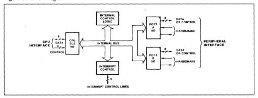
Figure 4: Typical Port I/O Block Diagram.
