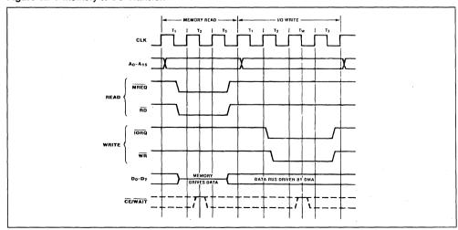
other T-cycle is added, during which the  $\overline{\text{CE}/\text{WAIT}}$  line will again be sampled. The duration of transactions can thus be indefinitely extended.
