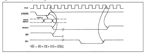
Figure 15: Mode 2 Bidirectional Timing.
