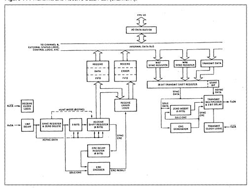
Figure 14: Transmitt and Receive Data Path (channel A).
