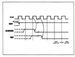
Figure 17: Bus Release at End of Block (Burst and Continuous Modes).
