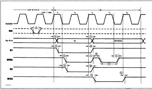
Figure 9 : Non-Maskable Interrupt Request Operation.
