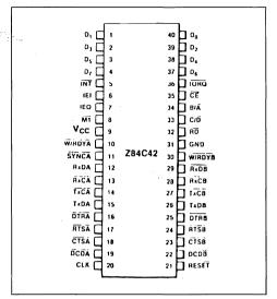
Both pins are Schmitt-trigger buffered to accommodate slow-risetime signals. The SIO detects pulses on these pins and interrupts the CPU on both logic level transitions. Schmitt-trigger buffering does not guarantee a specific noise-level margin.
