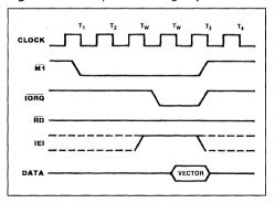
Figure 5d: Return from Interrupt Cycle.
