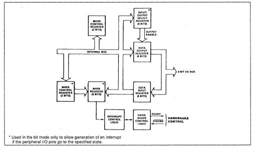
bits of the pointer. Each port (A and B) has an independent interrupt vector. The least significant bit of the vector is automatically set to 0 within the PIO because the pointer must point to two adjacent memory locations for a complete 16-bit address.
