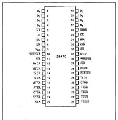
Figure 2: Chip Carrier Pin Configuration.
