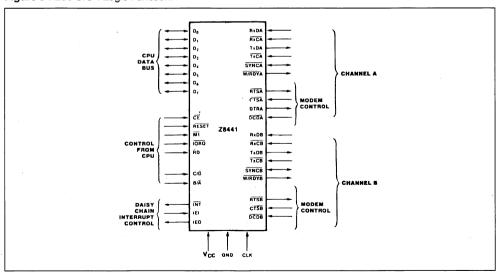
Figure 4 : Z80 SIO-I Dual in Line Pin Configuration.
