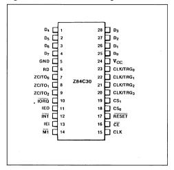
Figure 2: Chip Carrier Pin Configuration.
