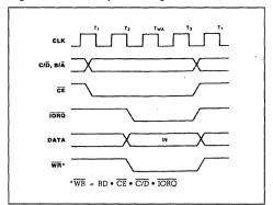
Figure 12: Read Cycle Timing.
