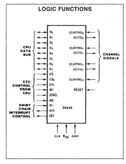
Figure 1: Dual in Line Pin Configuration.
