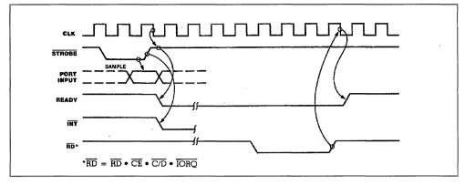
Figure 15: Mode 2 Bidirectional Timing.
