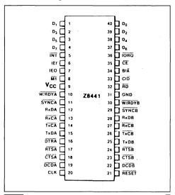
IORQ are all active, the channel selected by B/A transfers data to the CPU (a read operation). When CE and IORQ are active but RD is inactive, the channel selected by B/A is written to by the CPU with either data or control information as specified by C/D. If IORQ and M1 are active simultaneously, the
