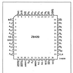
A and Port B. Each port has eight data bits and two handshake signals, Ready and Strobe, which control data transfer. The Ready output indicates to the peripheral that the port is ready for a data transfer. Strobe is an input from the peripheral that indicates when a data transfer has occured.
