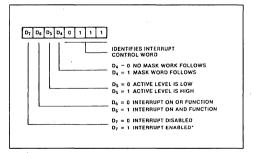
another control word that sets the I/O control register, which in turn defines which port lines are inputs and which are outputs (figure 7).
