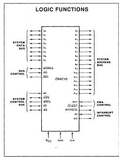
Figure 1: Dual in Line Pin Configuration.
