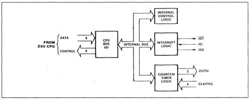
Figure 4: Counter/ Timer Block Diagram.
