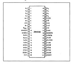
Figure 7: Chip Carrier Pin Configuration.
