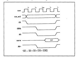
Figure 13: Mode 0 Output Timing.
