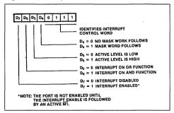
MASK CONTROL WORD. This word sets the mask control register, allowing any unused bits to be masked off. If any bits are to be masked, then D<sub>4</sub> must be set. When D<sub>4</sub> is set, the next word written to the port must be a mask control word (figure 9).
