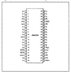
Figure 2: Chip Carrier Pin Configuration.
